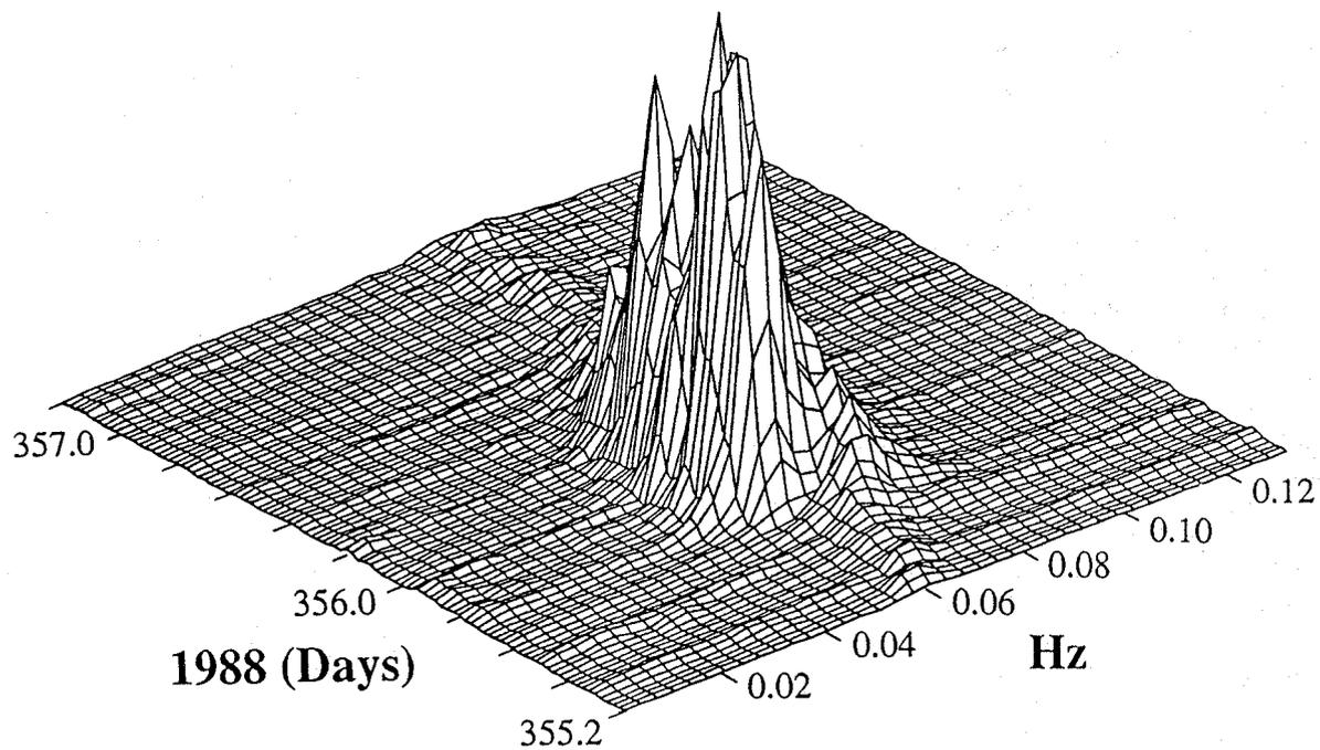
Figure 2. Spectrum of shelf floor pressure computed *in situ* from 1.67 Hz measurements transformed by integer FFT every 30 minutes.
