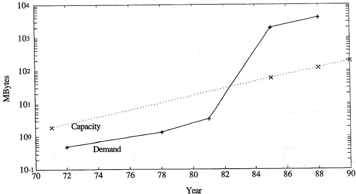
Figure 1. Williams' demand for data capacity vs. available underwater logger capacity. Demand outpaces supply. Data compression is required.
