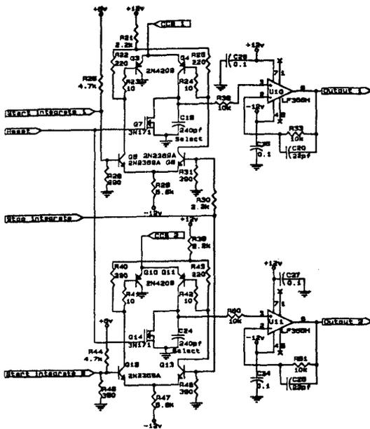
Fig. 1 Differential time to voltage circuit. Dual integrator.
