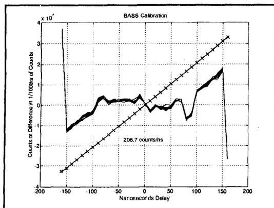
Fig. 4 BASS calibration with fast constant current source. The maximum difference between observations and their linear fit is 1/3%. Ten observations are plotted per delay and this appears to thicken the curve of differences.
