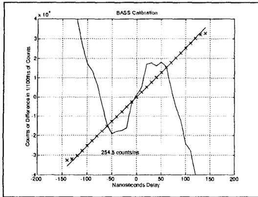
Fig. 2 BASS calibration with the slow constant current source. The straight line is a linear fit, Xs are measured observations, and the curved line is the difference between the observations and the linear fit magnified by 100.
