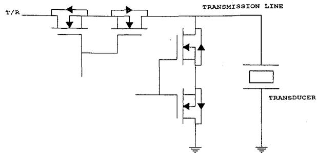
Figure 3. QUAD FET L-SECTION - The shunt and series portions of the L-section are each composed of two FETs connected source to source. This arrangement prevents halfwave rectification of the signal by the drain-source diode of the "open" branch of the L.
