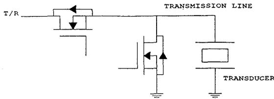
Figure 2. FET SHUNT SWITCH - The series and shunt FETs are operated in opposite states. The shunt switch is used to eliminate capacitive feedthrough coupling when the series switch is open. It has the added benefit of strongly reducing acoustic coupling by connecting the signal terminal of the deselected transducer to ground through the transmission line.
