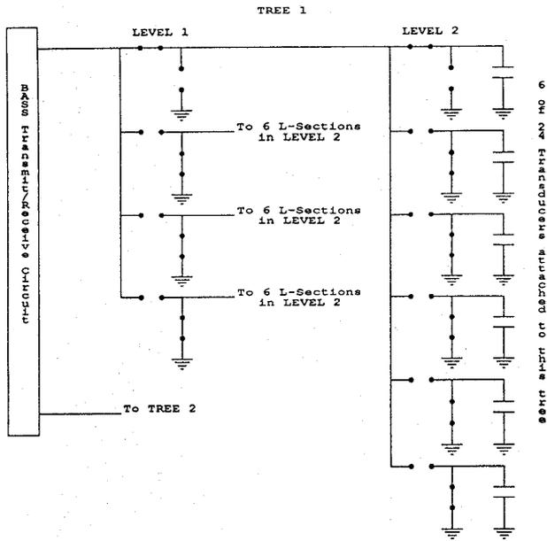
Figure 4. TWO LAYER MULTIPLEXER - The tree structure hides a portion of the capacitive shunt load behind deselected L-sections. The arrangement shown is optimal for a single T/R board. The FET L-sections are drawn as a pairs of switches and only a portion of the first tree is shown for simplicity. The upper L-sections in each level of the first tree are selected. One L-section in each level of the second tree, not shown, is also selected. All other L-sections in both trees are deselected.
