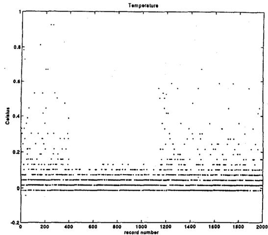
Fig. 4. Temperature sampled at 4 Hz in an icebath from a Sea-Bird temperature sensor.
