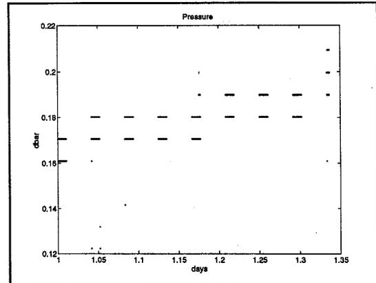
Fig. 2. Pressure from a Paros Digiquartz sensor the frequency of which was multiplied by 32 in a phase-locked-loop and sampled at 4 Hz by shifting the accumulated 24 bit count out of a serial shift register. Overscaling was restored by the algorithm above.
