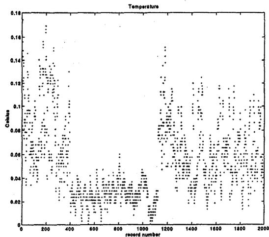
Fig. 5. The data of Fig. 4. averaged over ten points to give a tenfold improvement in resolution with 2.5 second temporal resolution.
