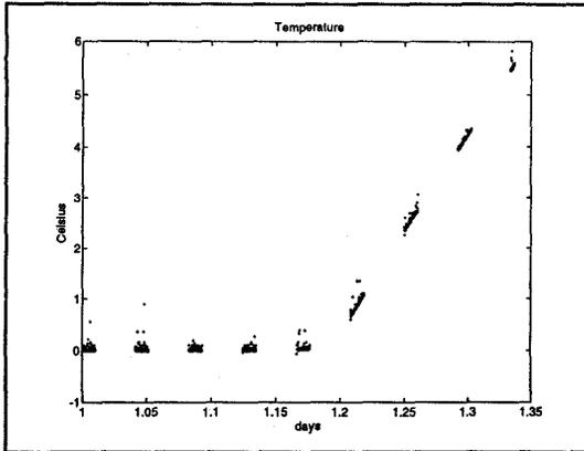
Fig. 3. Temperature from two Sea-Bird sensors sampled at 250 ms in a stirred ice bath. When the ice melted, both sensors tracked the warming water. Multiple overscalings of the counter between strobes occurred.
