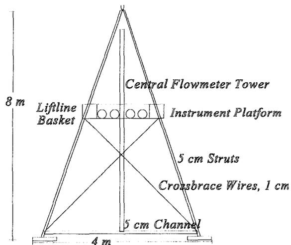
Fig. 3. SuperBASS tripod supports a tower of acoustic current meters (BASS) from 30 cm above bottom to 7 meters above bottom. To minimize turbulent wakes at the sensing levels, the faces are open, stiffened with crossbrace wires. The feet are held (as well as the bottom of the BASS tower) by a "Y" channel
