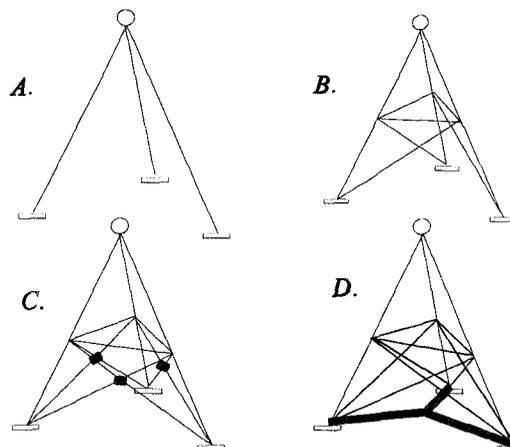
Fig. 1. A. Primitive tripod with feet fixed by seafloor. B. Tripod with platform attached to the struts at an intermediate position. Diagonal stiffening struts are required to regain stiffness of the tripod. C. Crossed stiffening struts to position feet during handling, before making contact with the seafloor. Intersection of the diagonal stiffeners blocks flow. D. Cable stiffened face of open tripod for minimum flow obstruction with "Y" box channel to position feet during handling.
