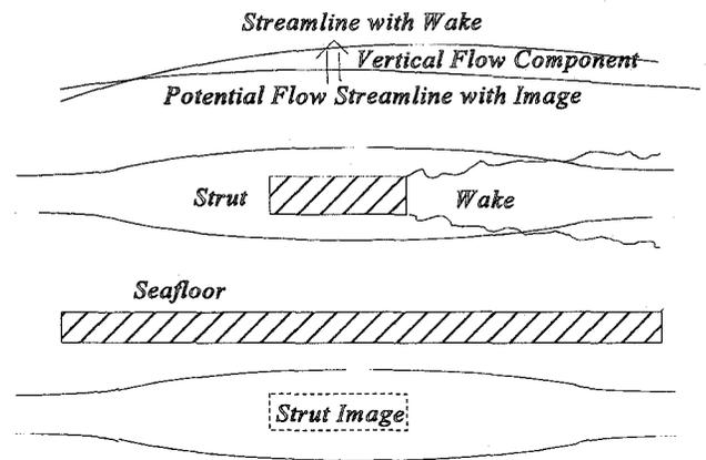
Fig. 2. The rectangular strut separating feet produces potential flow distortion accelerating the streamwise velocity but also producing a vertical component of velocity for any flow direction. The bottom distorts the flow as well, represented in the figure as an image below the seafloor.
