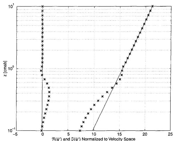
Figure 2. REAL AND IMAGINARY PARTS OF THE EIKONAL - The \*s mark the real and imaginary parts of the eikonal normalized to velocity space. The solid lines mark the logarithmic velocity profile and zero. Significant measurement bias exists only within millimeters of the bottom. The bias is systematic and could be removed in post-processing.
