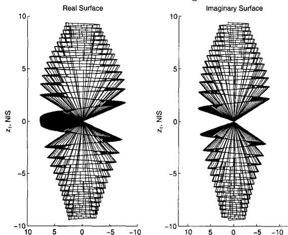
Figure 1. REAL AND IMAGINARY PARTS OF THE EIKONAL INTEGRAND - This is an NIS end view along the centerline with the transducers  $5 \text{ cmab}$ . Note the mild asymmetry caused by the changing curvature of the logarithmic velocity profile. The rapid oscillations of the exponential, the mathematical manifestation of the concentric Fresnel shells, and the relative importance of the central portion of the Fresnel pattern, the effective sample volume, are readily apparent.
