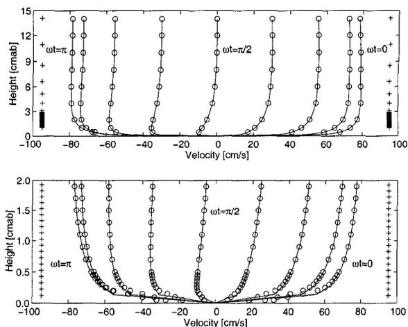
Figure 5. IMAGING A TURBULENT WAVE BOUNDARY LAYER WITH 5 MHz, 2.5 mm TRANSDUCERS - Detailed, accurate measurements of the vertical structure of a turbulent continental shelf wave bottom boundary layer could be made with these transducers. The notation is defined in the caption of the previous figure.
