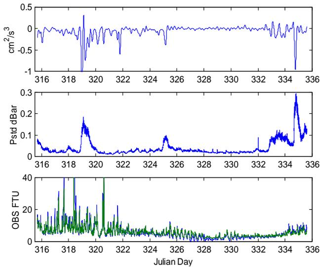
Fig. 11. The top graph is TKE generation minus dissipation in half-hour means for the entire deployment for the top sensor. The middle and bottom graphs show pressure standard deviation, a proxy for waves, and optical backscatter, a proxy for stratification by sediment load. Some negative correlation is seen between the excess TKE and pressure standard deviation.
