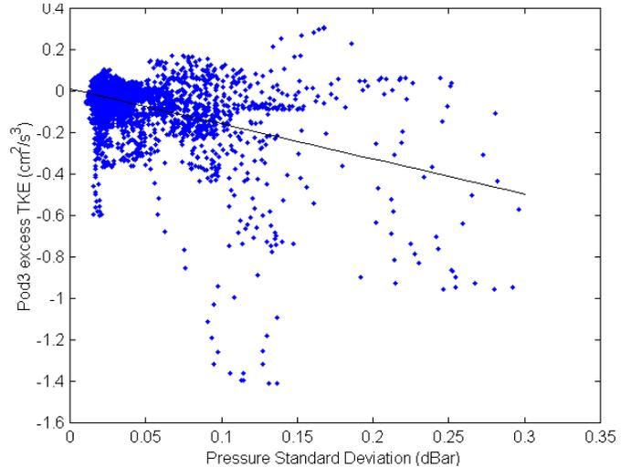
Fig. 12. Scatter plot of TKE generated by mean shear minus dissipation plotted against pressure standard deviation, a measure of wave activity.
