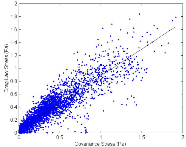
Fig. 5. Scatter plot of seven-minute means of drag-law stress to the half-hour means of covariance stress both from the middle sensor, showing good correlation.
