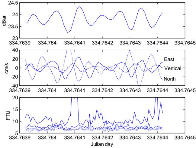
Fig. 2. North Sea BASS short time record of absolute pressure, velocity of sensor three, and optical backscatter at five heights above bottom.
