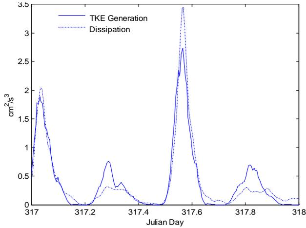
Fig. 10. Time record of half-hour means of turbulent-kinetic energy generated by mean shear and dissipation.
