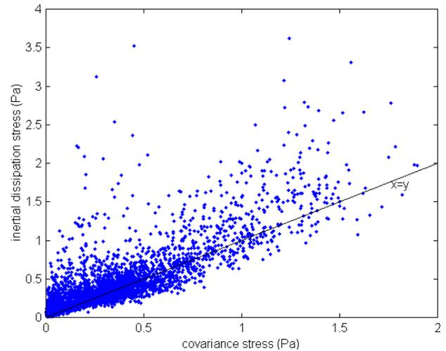
Fig. 8. Scatter plot of seven-minute means of inertial dissipation stress to half-hour means of covariance stress.
