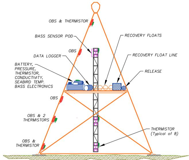
Fig. 1. BASS tripod configuration used the North Sea deployment.
