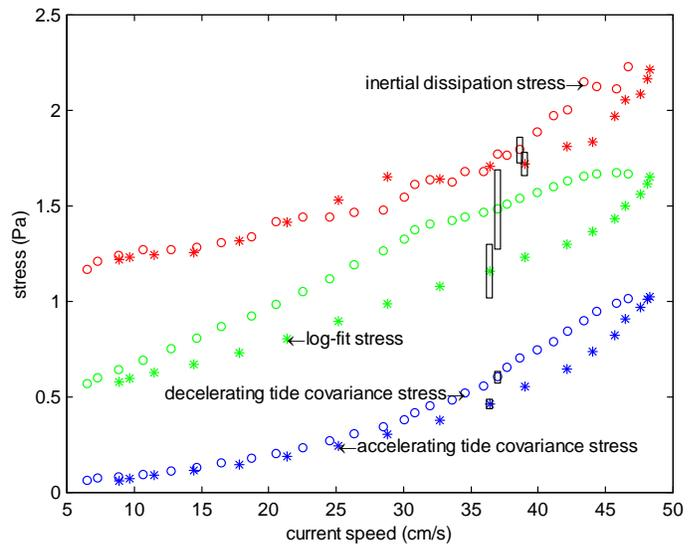
Fig. 9. Current velocity and stress estimates from covariance, log-fit displaced up by 0.5 Pascals, and inertial-dissipation displaced up by 1 Pascal, of the first half of the average of 38 semidiurnal tidal cycles. The rectangles represent the 95% confidence intervals due to statistical variability of current, covariance and inertial dissipation stresses and the 90% confidence interval for the log-fit stress.
