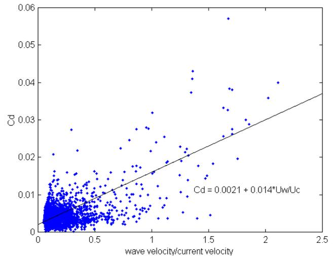
Fig. 6. Scatter plot of half-hour computed drag coefficient from the covariance stress and mean velocity plotted as a function of the wave velocity divided by the current, when the current exceeded 5 cm/s.
