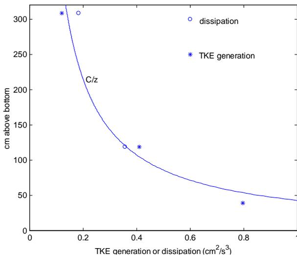
Fig. 13. Means for the entire deployment of TKE generated by mean shear and dissipation. The line is a wall-layer model fitted to the generation of the upper two sensors. The data balances generation and dissipation to within the standard error.
