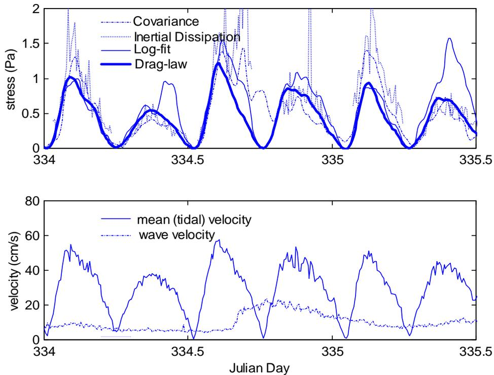
Fig. 4. The top graph is a time series, during a storm, of stress estimates from the drag-law, covariance, log-fit, and inertial dissipation methods. The lower graph is a time series of mean velocity (mostly tidal) and wave velocity. During the peak of the largest storm the covariance stress estimate diverged from the other estimates when the wave velocity was more than four times the mean velocity.
