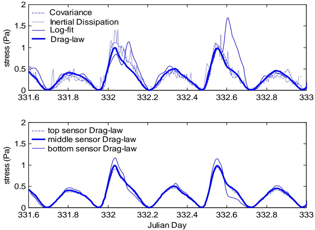
Fig. 3. Time series of stress estimates from drag-law, covariance, log-fit, and inertial dissipation methods. The period in the top graph when the log-fit stress diverged from the other estimates corresponds to a period of reduced measured flow by the bottom sensor, shown by the lowered bottom sensor drag-law stress.
