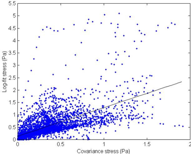
Fig. 7. Scatter plot of half-hour means of log-fit stress to the half-hour means of covariance stress.
