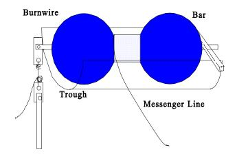
future deployments will use a horizontal cradle of 19 cm PVC pipe, split in half. One end of the shaft through the float will be tucked under a bar and the other end will be held down by the burnwire as in Fig. 5. This geometry lowers the profile and resists fouling by marine organisms and sediment. PVC will not corrode or influence the burnwire corrosion current at release time.
