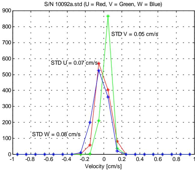
Fig. 2, Histogram of instantaneous velocity measurements in a still bucket over 10 minutes. The electronic noise level is 0.056 cm/s and the velocities are only slightly more than that.
