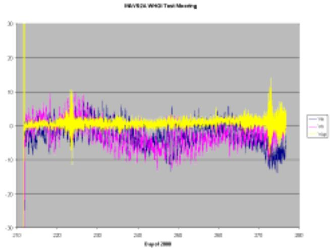
Fig. 8. Moored MAVS at 2000 m near Bermuda. Sampling at 5-minute period, vertical velocities of 10 cm/s amplitude are seen at day 224 and day 273 lasting about 8 hours each time.
