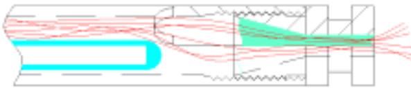
Fig. 4. The original MAVS sensor tube has an epoxy pressure block in the tapered plug and urethane water block surrounding the enameled copper wires and urethane pressure compensation tube. The epoxy is indicated with fill in this drawing. The closed end of the pressure compensation tube approaches the tapered plug but it does not touch the epoxy.
