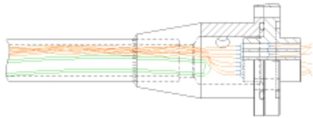
Fig. 5. Hermetic sealed feedthrus provide the pressure block in the new MAVS sensor tube. Urethane serves as a water block. A pressure compensation tube extends nearly to the end of the urethane to prevent longitudinal strain from breaking the wires.
