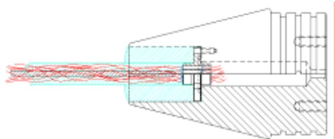
Fig. 6. Endoskeleton version of sensor support with flexible outer skin to reduce stresses in the urethane bond to the wires and pressure blocking feedthrus.
