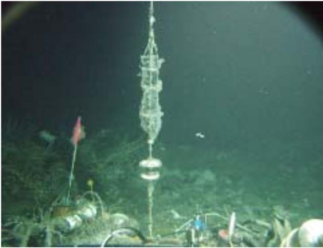
Fig. 3. MAVS current meter at 2300-m depth at the Endeavour Field of the Juan de Fuca hydrothermal vent field. Photograph from DSRV Alvin.
