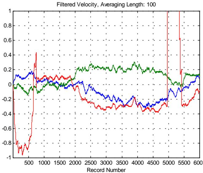
Fig. 7. Zero velocity offset dependence on pressure. MAVS sensor cast in solid carrageenan gel during a lowering to 1000 m and return. The net change in offset was about 0.1 cm/s but at 100 bars the offset was about 0.3 cm/s.
