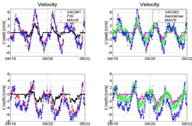
Fig. 7. Four-day section of record to show typical stalling of both VACM sensors
