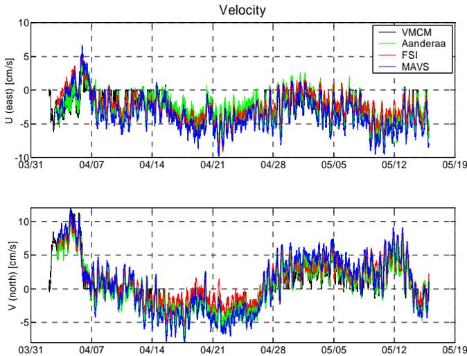
Fig. 9. Velocities measured by the four instruments in Ultramoor 2002
