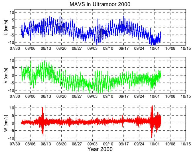
Fig. 1. Two-month record from Modular Acoustic Velocity Sensor sampling at 5 minute intervals at 2000-m depth in 4000 m water depth east of Bermuda.
