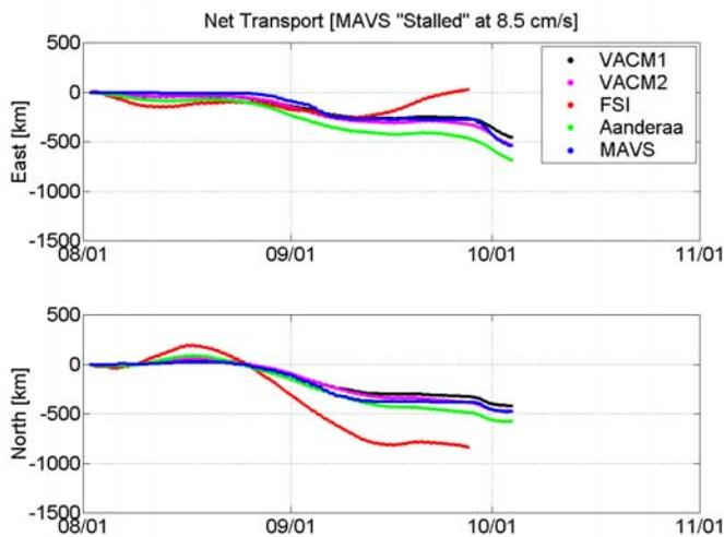
Fig. 6 Net transport as in Fig. 5 but with MAVS "Stalled" below 8.5 cm/s
