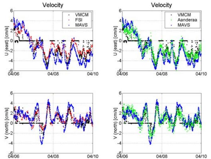
Fig. 11. Four-day section of record with typical stalling of VMCM sensor
