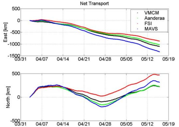
Fig. 10. Integrated velocities from four instruments. The scale in the North plot is expanded.
