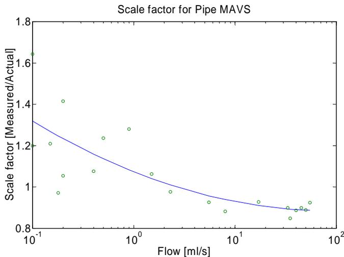
Fig. 9. Ratio of integrated flow to total volume
