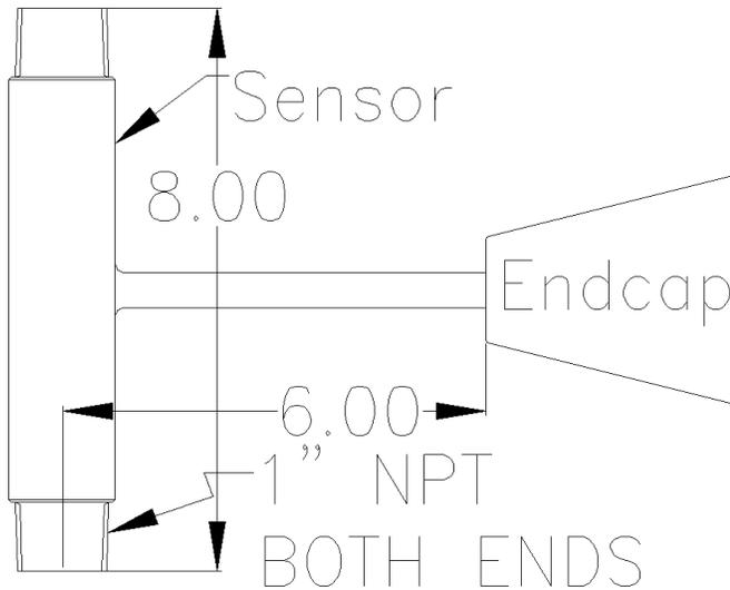
Fig. 1. Pipe sensor on endcap, dimensions in inches
