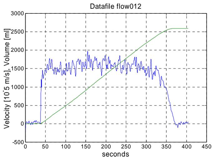
Fig. 8. Integrated flow measurement for 2440 ml. Sloped line is volume
