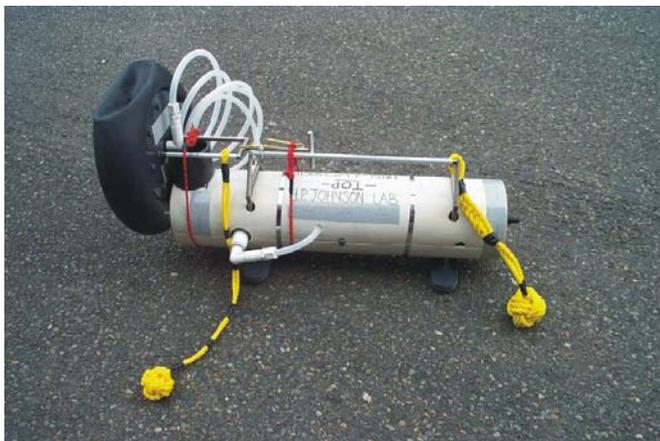
Fig. 10. Field deployable Pipe MAVS in PVC housing with titanium handle for deployment by ROV
