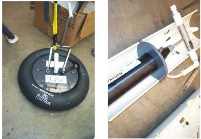
Fig. 11. Innertube collector filled with dense saline solution on the left and Pipe MAVS with hose in PVC case on the right. T bar handle permits ROV to position the collector over a diffuse hydrothermal vent.
