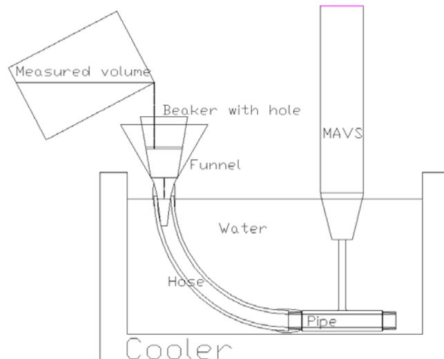
Fig. 7. Pipe MAVS calibration bath
