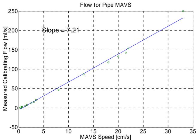
Fig. 5. Calibration of Pipe MAVS with continuous flow
