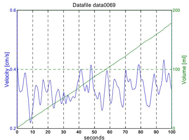
Fig. 4. 0.48 ml/s flow. Sloped line is volume
