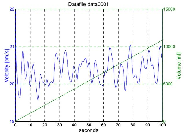
Fig. 3. 133.3 ml/s flow. Sloped line is volume
