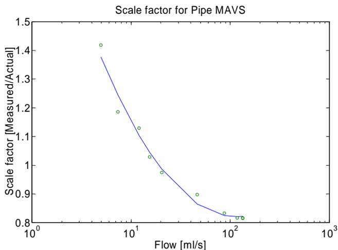
Fig. 6. Ratio of flow measured in Pipe MAVS to actual flow
