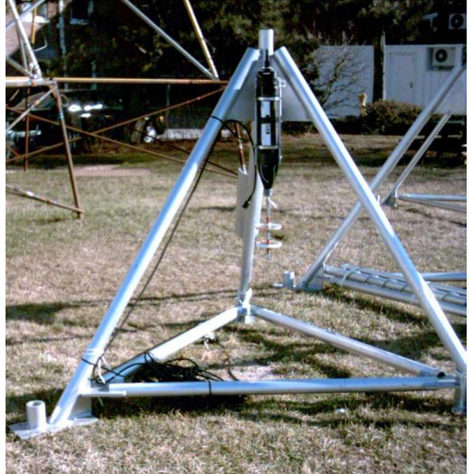
Fig. 8. One of two tripods with MAVS sensor to observe the vector velocity and pressure at 0.75 m above the bottom.
