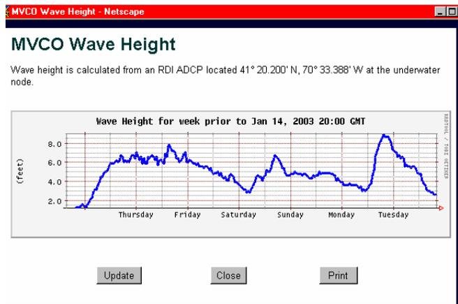
Fig. 7. Processed data from a computer logging files at the shore station.
