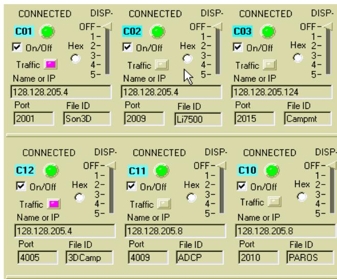
Fig. 4. SPIPTCP1 Lab View screen to enable logging serial data streams in the scientific laboratory or remotely at the shore station.
