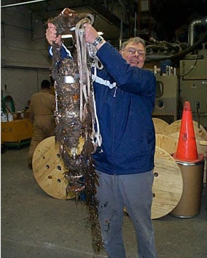
Fig. 11. MAVS recovered after two months at 2 meters depth. Acoustic current measurements had stopped due to fouling.
