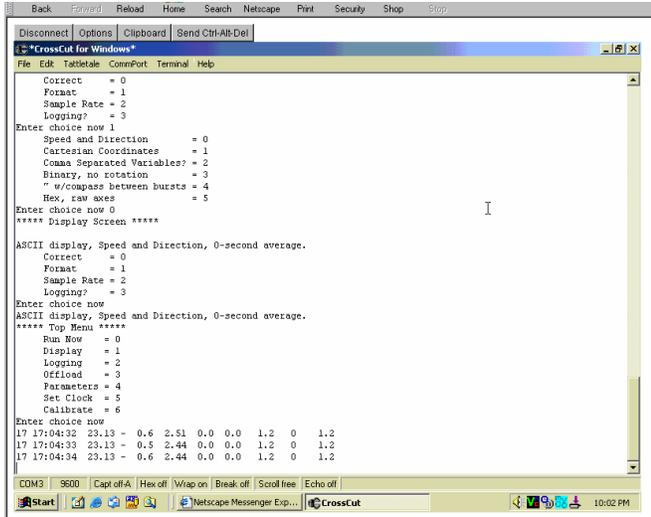
Fig. 5. Transaction between computer in the lab and a MAVS2 current meter on a network mediated with VNC Desktop under Internet Explorer.
