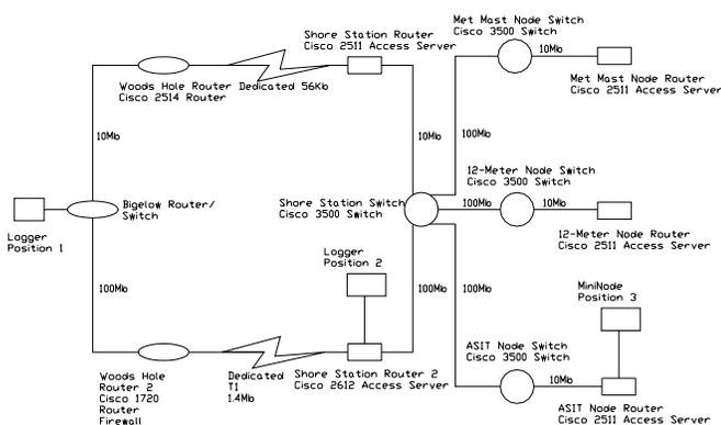
Fig. 3. MVCO Network Configuration, courtesy John Krauspe, Woods Hole Oceanographic Institution.
