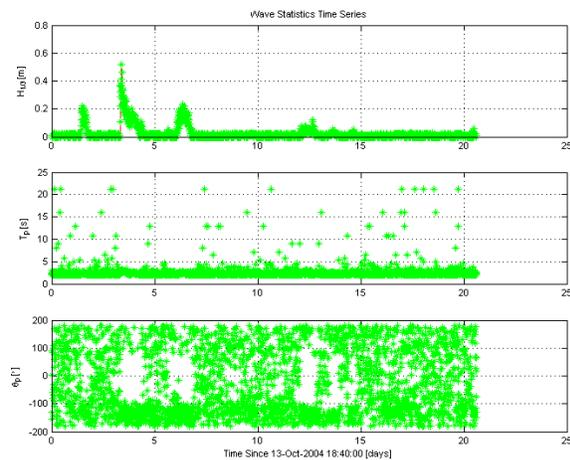
FIGURE 11 – MWAVES time-series showing the statistical evolution of the wave field in Polson Bay during the second deployment, October 13 to November 8, 2004. Significant wave height exceeded 0.5 meters at 03:50 on October 17, 2004. The spin-up time from flat calm conditions to this peak was only 90 minutes. The relaxation time was over a day. Such strong, sudden onset events are not uncommon.
