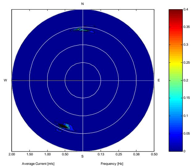
FIGURE 5 – MWAVES directional wave spectrum for 20:00 on September 30, 2004. This was the time of greatest significant wave height during the first deployment. The plot indicates that 2.8 second waves were propagating to the south-southwest, reflecting off the wall at the south end of the lake, and propagating back to the north.
