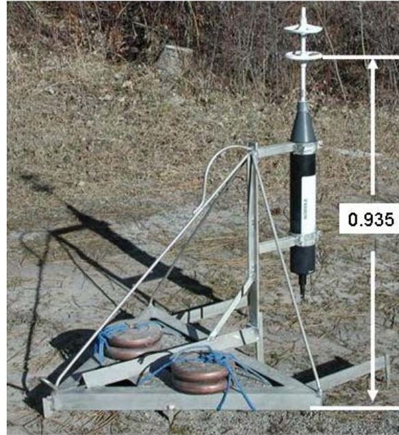
FIGURE 3 – MAVS on the Flathead Lake Bottom Frame. The height of the MAVS velocity sensor is 0.94 m above the bottom. The pressure sensor in the conical end cap is 0.68 m above the bottom. The frame was deployed in 3.5 m depth on a flat bottom in Polson Bay.
