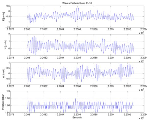
FIGURE 10 – Two minute record, one burst, from the wind wave event of November 10, 2004. The event lasted for 10 hours beginning at elapsed hour 65 in Figure 9. Unfiltered velocity measurements show a north-south component of wave velocity with a 1 cm/s amplitude and a 2.17 second period. While the significant wave height,  $H_{1/3}$ , briefly reached 8 cm during this event, it was probably no greater than 2 to 4 cm when this burst was recorded.
