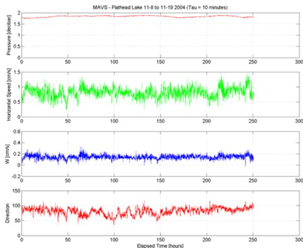
FIGURE 9 – MAVS data for the third deployment after smoothing with a 10 minute Butterworth filter. The filtered data show low frequency variations in pressure of about 0.1 dbar, a depth change of ~10 cm. No average velocities greater than 1 cm/s were observed.
