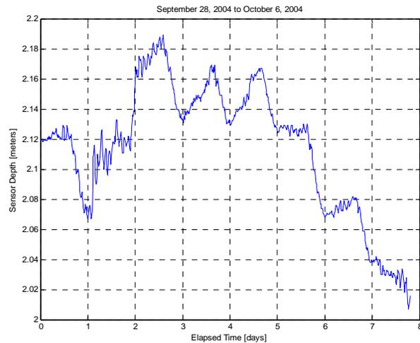
FIGURE 6 – Pressure Time-Series. The MAVS pressure record for the first deployment, which began on September 28 at 19:30, is shown in blue. Note the persistent diurnal signal, with minima in the evening and peaks in the morning. The 2 hour seiche is episodic and most clearly apparent between 2 and 2.5 elapsed days. Trends of longer duration are also present.
