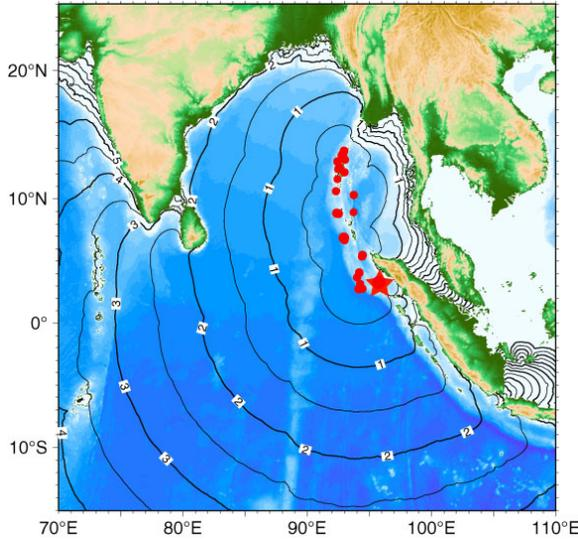
Fig. 1. December 26, 2004 Sumatran tsunami. Heavy lines are whole hour tsunami arrival times after the earthquake. The tsunami arrived at Banda Aceh in less than 20 minutes while it arrived at Sri Lanka two hours after the earthquake. From National Institute of Advanced Industrial Science and Technology.
