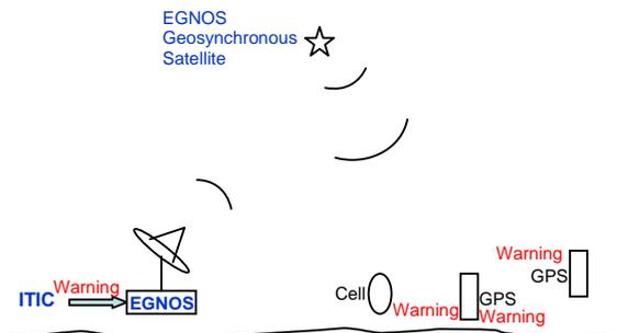
Fig. 7. ALIVE system for disaster prevention and mitigation. Warning is transmitted from ITIC and downloaded to geosynchronous satellite where it is transmitted as part of the SBAS (EGNOS, WAAS, or MSAS) GPS correction message. This message is received by GPS receivers and by cell phones equipped with GPS receivers (911 enabled).
