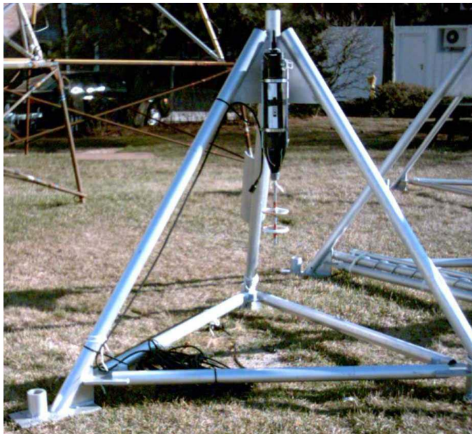
Fig. 7. Bottom tripod for wave and current measurements. The velocity measurement volume is 0.75 m above the bottom. The tripod is shown with a MAVS (Nobska Development, Inc.) current meter, mounted sensor down. Pressure is measured at a height of 0.85 m.
