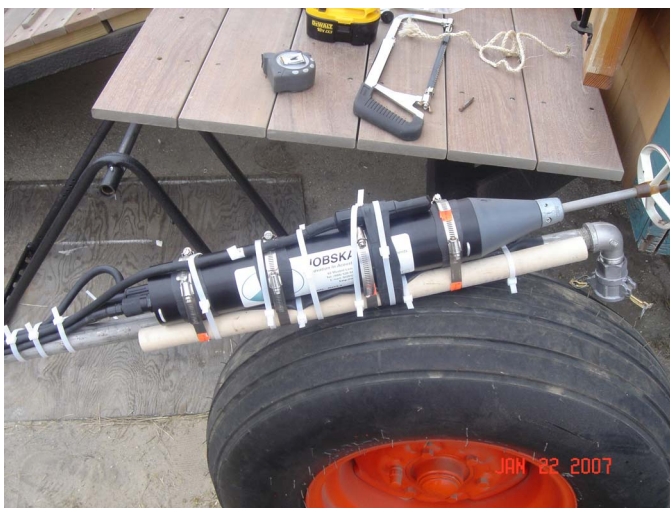
Fig. 5 MAVS current meter on pipe preparatory to jetting into the sand. The acoustic travel-time sensor is a pair of rings at the top (on the right in the photograph) where only the lower ring is visible.
