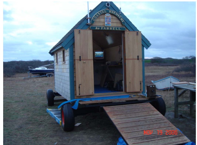
Fig. 3 Portable Research Lab on a trailer for emplacement at a beach to support the offshore instruments.
