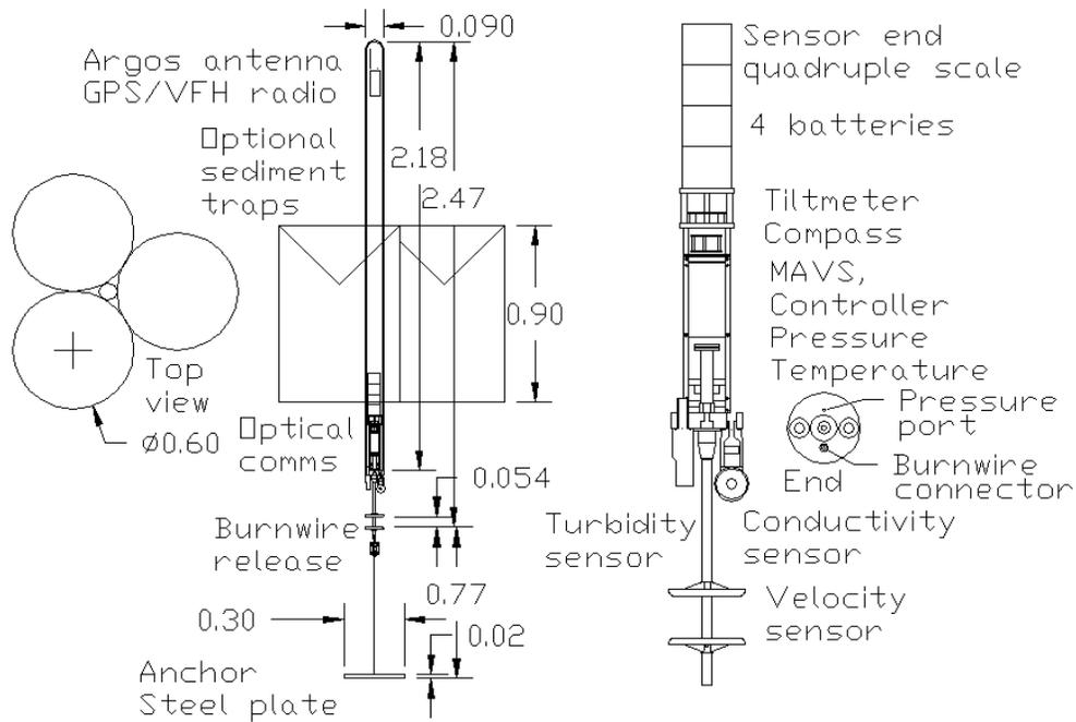
**Fig. 2. Down configuration for the XBL with steel plate anchor. The sensor volumes are  $\frac{3}{4}$  meter above the bed. As illustrated, all the sensors possible are included. Optional sediment traps can be clamped around the housing since the XBL does not invert when released.**
