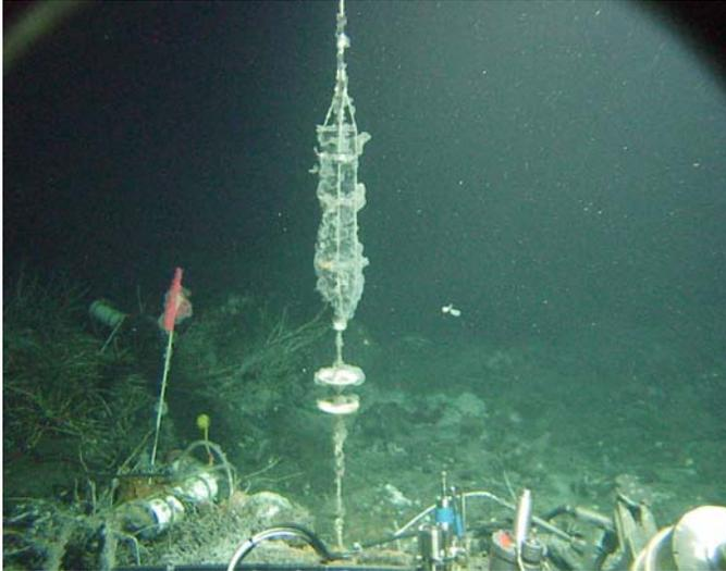
**Fig. 4. MAVS at 2300 meters at the Endeavour Field of the Juan de Fuca hydrothermal vents. Organisms growing on the sensor after 2½ months did not impede the measurement of the flow to any noticeable extent.**
