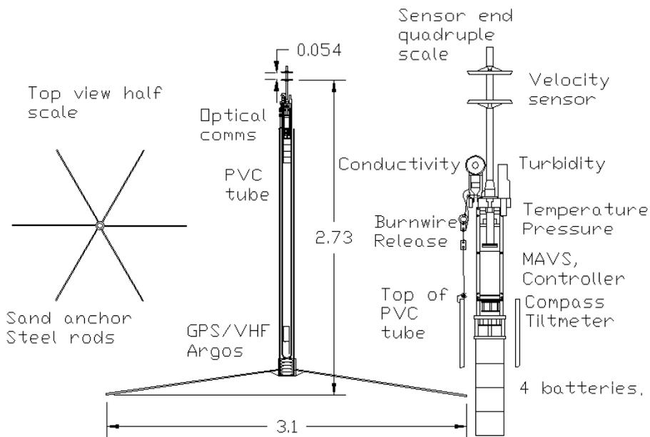
**Fig. 3. Up configuration of the XBL with sand anchor. The sensor volumes are  $2\frac{3}{4}$  meters above the bed. As illustrated, all the sensors possible are included although in use some or all of the optional sensors may be replaced with dummy plugs. A burn wire keeps the XBL in the launch tube until a preset time. The XBL inverts when it is clear of the tube and extends its antenna end above the surface for radio transmission.**
