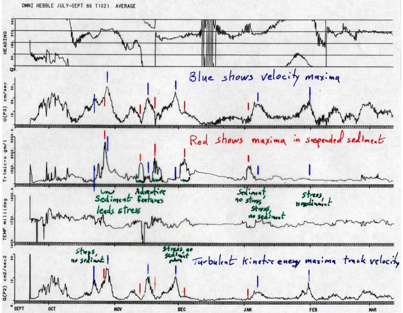
**Fig. 1.** BASS logged compact data show bottom current and speed, optical turbidity, temperature, and turbulent kinetic energy from 30-minute averages of 2-Hz samples. This display is derived from a single sensor of a six-sensor array over a 6-month deployment all stored in 2 Mbytes of memory.
