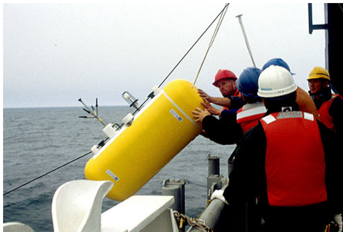
Fig. 2. McLane moored profiler being deployed.
