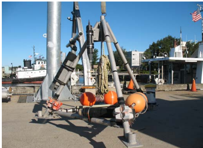
Fig. 4. Small tripod to support ADCP and MAVS current sensors with Pop-Up floats for instrument recovery carrying Spectra line.
