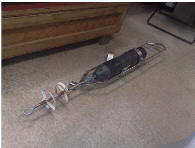
Fig. 1 MAVS current meter is displayed in an early mooring frame that carries tension around the electronics housing to the sensor tube where it is carried in the stainless steel tube to an eye bolt at the end of the sensor. The two rings support 8 acoustic transducers that define the four oblique measurement axes along which components of the flow are measured. Except for reduction in housing size, the mechanical configuration of MAVS has changed little.
