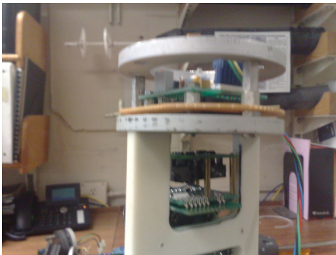
Fig. 4. MAVS2 is shown here with a gimballed two-axis magnetometer compass and a fluid-filled tilt meter above the compass.
