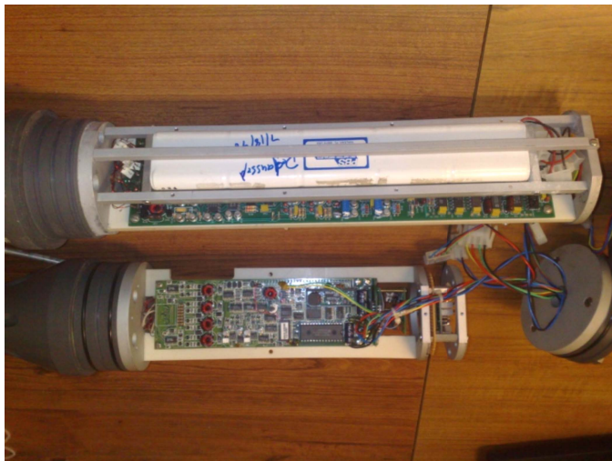
Fig. 3. MAVS 1 is shown above and MAVS2 beneath as in Fig. 2 but with each chassis inverted. The battery of 15 AA cells is visible on the back of MAVS 1 beneath an aluminum bar. Part of the MAVS 1 circuit board is visible above the thick plastic chassis. It is almost double the size of the MAVS2 circuit board that uses surface mount chips rather than the leaded parts of MAVS 1.
