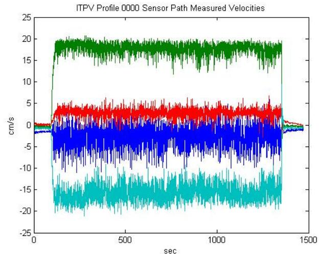
Fig. 2. Sensor path velocities from the first down-going profile of the ITPV deployment are plotted. The blue path is downstream of the sensor and has the most noise, and the red path is the upstream path with the least noise.
