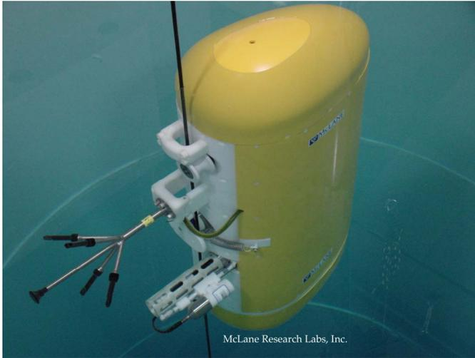
Fig. 3. McLane Moored Profiler with Falmouth Scientific Instruments acoustic current sensor in McLane test tank. Courtesy of McLane Research Inc.
