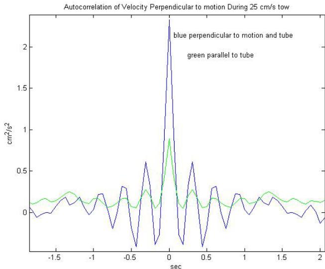
Fig. 12. The autocorrelation of 16 Hz velocity normal to carriage motion from tow-tank test is shown.
