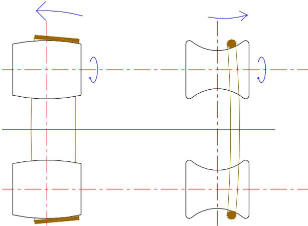
Fig. 7. Pulleys for belting are crowned to keep the belts centered on the pulleys. The shape of the ITPV guide rollers may cause the cable to climb out and then suddenly slide back shaking the profiler.
