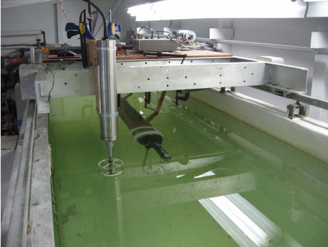
Fig. 9. ITPV and a MAVS are shown in the WHOI tow tank. The ITP is on the right and MAVS is on the left.
