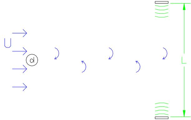
Fig. 8. A schematic of a vortex street in the wake of a bluff body advecting through the sensing volume of a travel-time current meter is shown.
