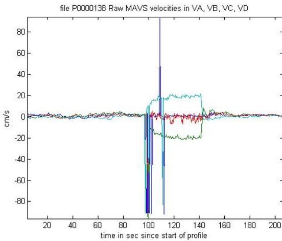
Fig. 5. An example is displayed of dropout in the measured path velocities during the switching "soft start" of the profiler. Shown are time series of the four MAVS velocity paths during a vertical profile in a test tank. The vehicle began to move around time 95 seconds and reached steady state profile speed around time 115 seconds. The vertical motion of the instrument ended around time 140 seconds, followed by a two minute sampling when the vehicle was stationary.
