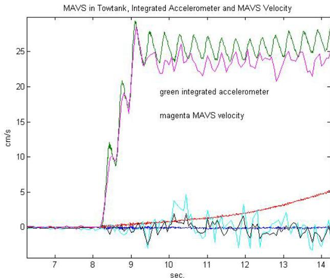
Fig. 10. Tow Tank velocity measured by a MAVS sampling at 16 Hz and deduced from time integration of data from a three-axis accelerometer is displayed. The along-carriage velocity estimates (green and magenta) show reasonable agreement. The blue, cyan, black, and red lines are velocities perpendicular to the carriage motion.
