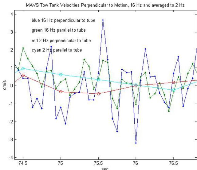
Fig. 13. Over-sampling and averaging in the time domain is demonstrated.
