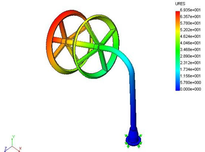
Fig. 4. Finite element vibration model of the sensor structure gave a lowest normal mode frequency of 34 Hz. The color shading indicates the amplitude of the resonant vibration.
