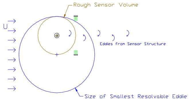
Fig. 11. The dominant eddies from the sensor structure are too small for the sensor to resolve. In this sketch, the small black circle can be thought of as the cross section of the sensor tube, the brown circle is a simplification of the sensing volume, and the blue circle is the size of the smallest eddy spatially resolvable with the sensing volume.
