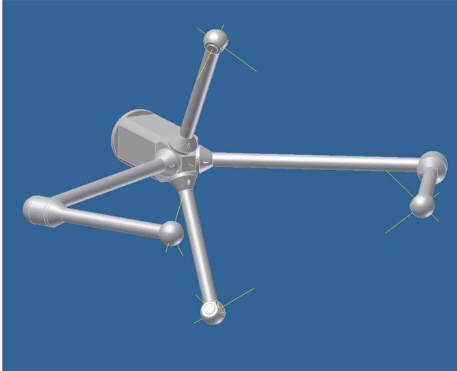
Fig. 15. Concept of an acoustic travel time sensor that is optimized for a profiler that orients into the incident horizontal flow is shown.
