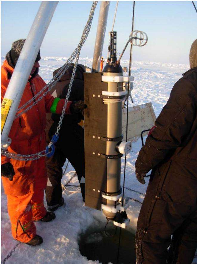
Fig. 1. Deployment of the first ITPV is shown. A tripod was used to support the wire tether and profiler during deployment. The MAVS acoustic current sensor supports are the circular rings extending up and to the right of the ITPV top end cap in this image. Black plastic tail fins extend off the trailing edge of the vehicle to orient the instrument into the relative horizontal flow.
