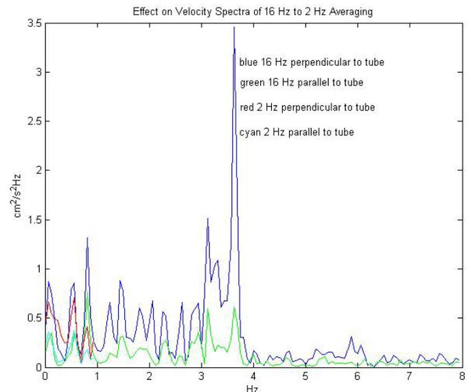
Fig. 14. Over-sampling and averaging in the frequency domain is illustrated in this figure. The blue and green lines are power spectra of the 16 Hz sampling and the cyan and red lines are spectra of the 2 Hz boxcar-averaged samples.
