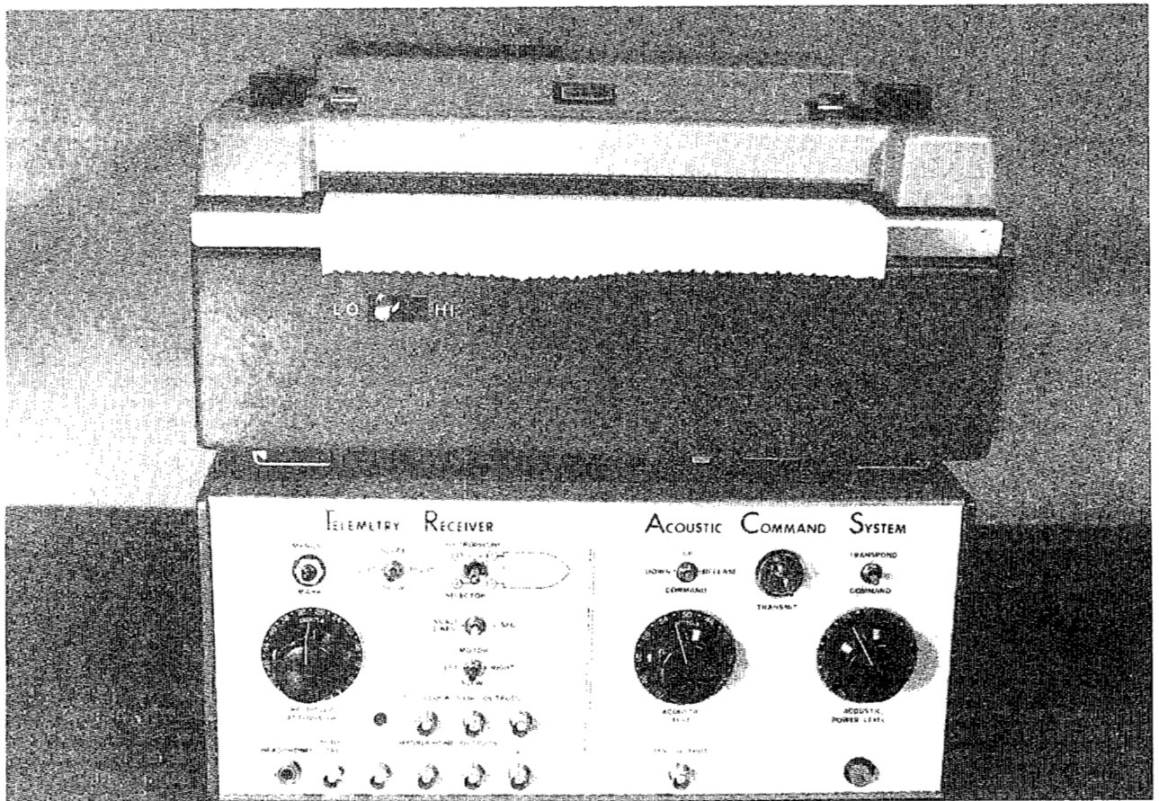
Figure 1. The Telemetry Receiver Acoustic Command System (TRACS) shown with the helix wet-paper recorder.
