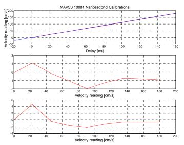
Fig. 5. Non-linear behavior of the MAVS3 used in the Intercomparison.
