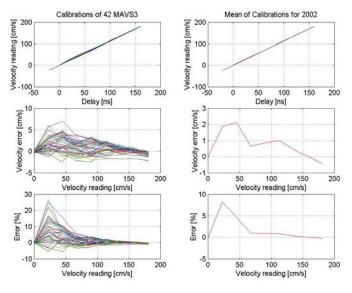
Fig. 4. Non-linearity of 42 MAVS3 instruments calibrated in 2002 with the average showing 8% over-reading near 20 cm/s.
