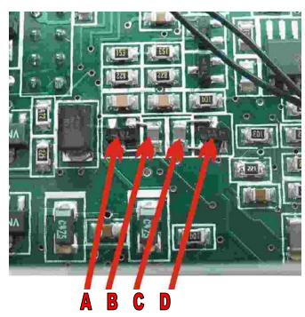
Fig. 10. A and D are RF NPN transistors that require "Miller" capacitors, B & C, for stability. However, without addition of short lengths of #26 bus wire visible between A & B and between C & D, ringing may occur producing non-linearity.
