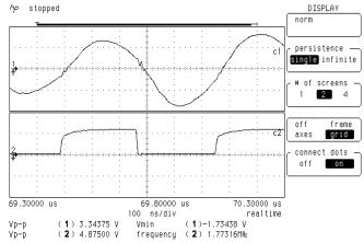
Fig. 7. 'Glitch' in received waveform in top trace when the voltage comparator output shown in the bottom trace changes state. This is a potential cause of non-linear behavior.
