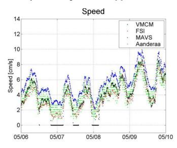
Fig. 2. Intercomparison of four current meters at 4000m depth near Bermuda where MAVS3 (in blue) is uniformly 1 to 2 cm/s higher than the mechanical VMCM, acoustic travel-time FSI, and acoustic Doppler Aanderaa. Note that the VMCM stalls below 2 cm/s.
