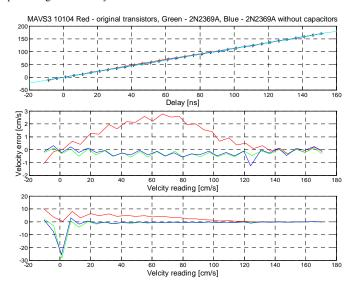
Fig. 11. Replacement of the RF NPN transistor with a 2N2369A NPN switching transistor removes non-linearity whether "Miller" capacitors are present or not. Electronic noise is also removed by this substitution.
