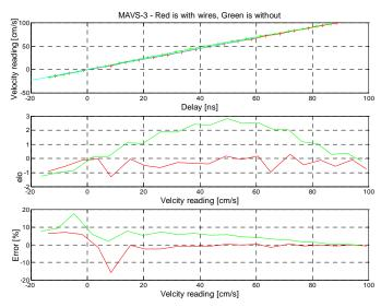
Fig. 9. Non-linearity is corrected with a short length of #26 bus wire laid on top of the 1/8" foil run to the "Miller" capacitor of the cascode transistor.
