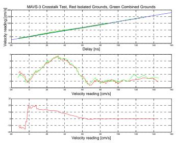
Fig. 8. Evidence that crosstalk from power and signal grounds are not the cause of non-linearity. The red curve results from separated grounds in which the 'glitch' of Fig. 7 is gone while the green curve results from common grounds where the 'glitch' is evident. There is no improvement due to separating the grounds.
