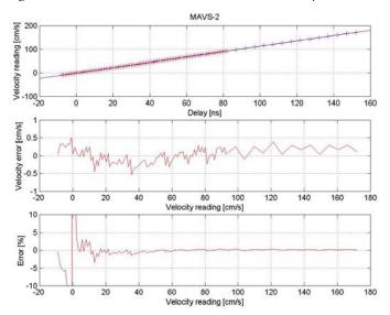
Fig. 6. Calibration of MAVS2 without evidence of non-linearity.
