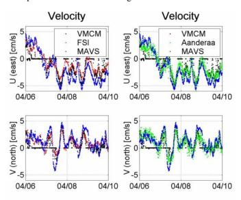
Fig. 3. Vector display of intercomparison of four current meters at lower flow rate than in Fig. 2. VMCM is stalled more often and the difference between the FSI, Aanderaa, and MAVS3 is reduced over that in Fig. 2.
