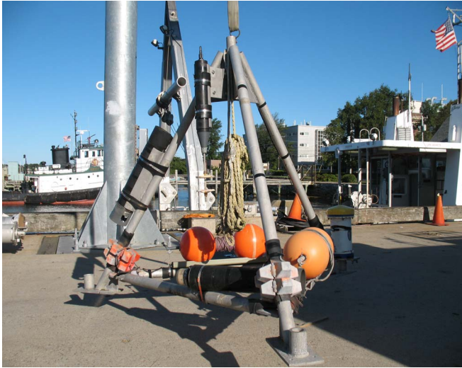
Fig. 1. The small tripod supports a MAVS and an ADCP sensor for current, wave, and turbulence measurements. The ADCP is on the far footpad, the MAVS is mounted to the vertex, and two acoustic command releases, one horizontal on the near strut and the other vertical on the left diagonal can activate the pop-up floats each with a pair of orange balls and a lift line wrapped around its axle.
