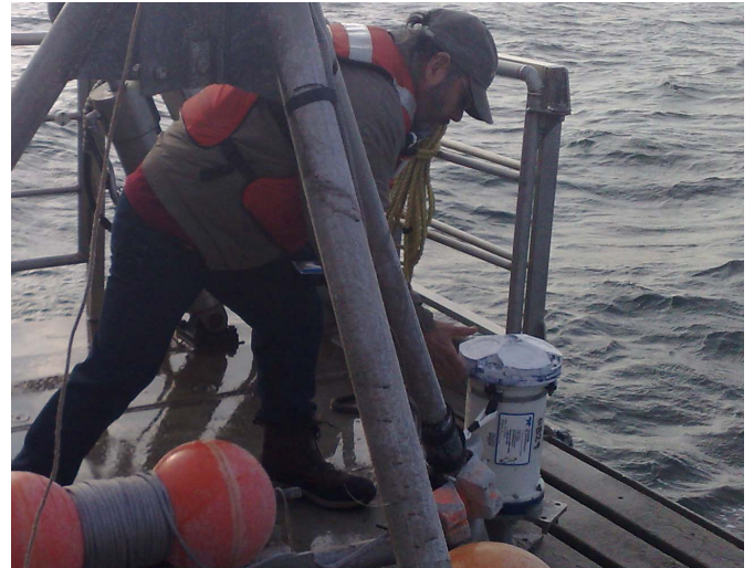
Fig. 2. The ADCP transducers are covered with Desitin™ to inhibit barnacle settlement.
