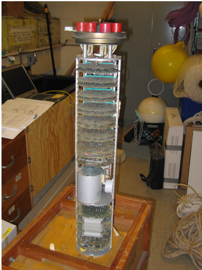
Fig. 3. BASS electronics rack based upon the electronics chassis design of Dick Koehler as introduced for the VACM with D-shaped circuit boards and the Elco 35 gold-plated contact connector. The VACM magnetically damped compass is the cylinder near the bottom. This BASS has an early microprocessor-based controller with a ribbon-connector bus giving it the designation of Smart BASS.
